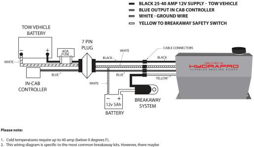
This wiring diagram is specific to the most common breakaway kits. However, there maybe different breakaway kits, which use other wiring configurations and color codes. Therefore, you will need to check the specific manufactures' specifications.
